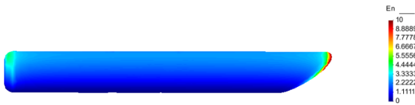
Fig. 3. Electric field E_n , normalized by the applied field, on the surface of R-S1 particle having the sharp tip separated from the electrode.
